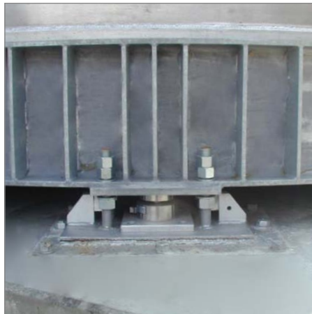
For a reliable control of the quantity of material inside the silos, it is possible to place the silo on load cells
