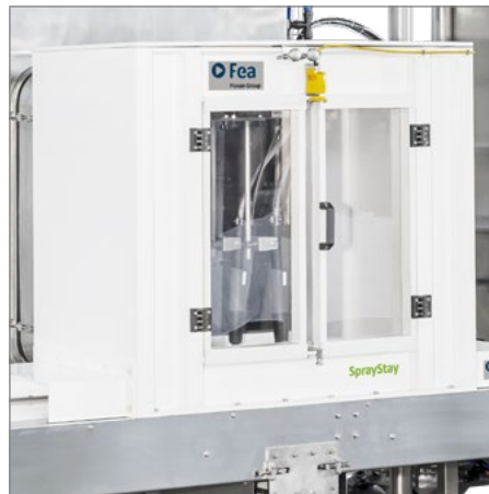
Powder containment booth in dielectric material with doors
