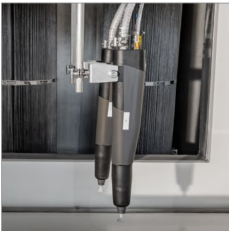
Electrostatic dispensers with interchangeable nozzle for different types of coverings
