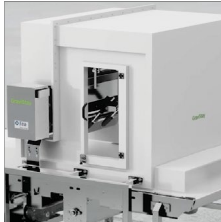
Powder dosing and electrostatic charging system inside the containment booth
