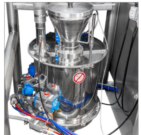
Powder tank in stainless steel with Venturi pumps for dosing and delivery to electrostatic dispensers
