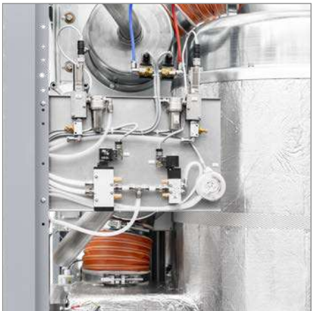
The Dew Point stabilizer (option) allows an advance control of the process, increasing stability level
