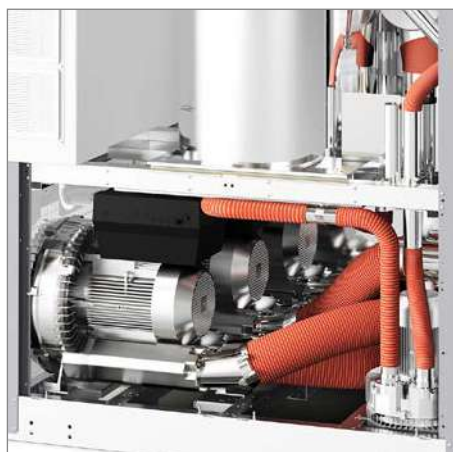
Process blower with on board frequency converter and Can Open communication interface to be fully integrated in the control
