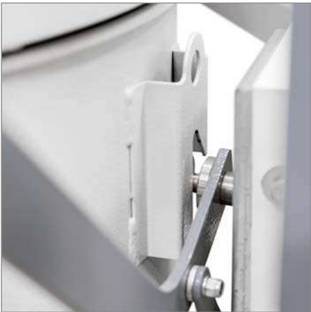
Lifting device to put in place the collecting bin and to easily connect it with the cyclone body (advanced bin)
