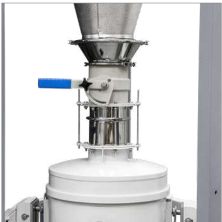
Manual valve to segregate the collecting bin from the process and to make possible the discharge operation without stopping the process
