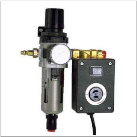
The control unit receives a signal from the sightglass sensor, which turns on the controller and supplies air to the venturi to move the material.
