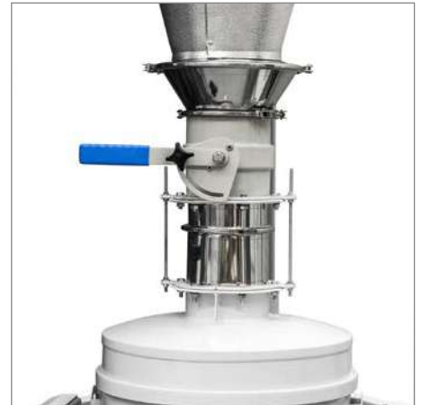
Butterfly valve to separate the collecting bin from the process
