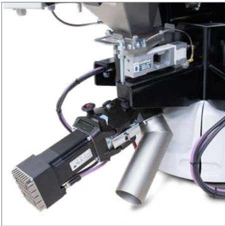
The entire dosing station is weighted by the load cell to ensure higher precision and accuracy
