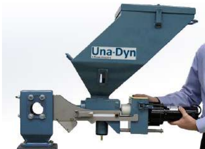
Release clamps on sides of gearbox motor
